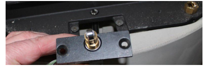
Illustration 55: Placing the door contact switch on the stove front transverse web
