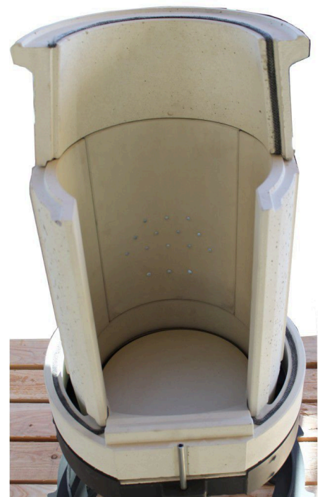
Illustration 17: Rear intermediate part laid and aligned
