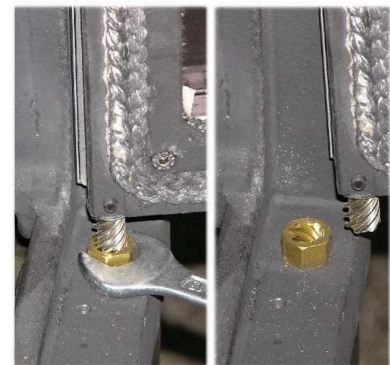
Illustration 26: Set the hinge bolt onto the threaded sleeve and adjust in height by turning the threaded sleeve
