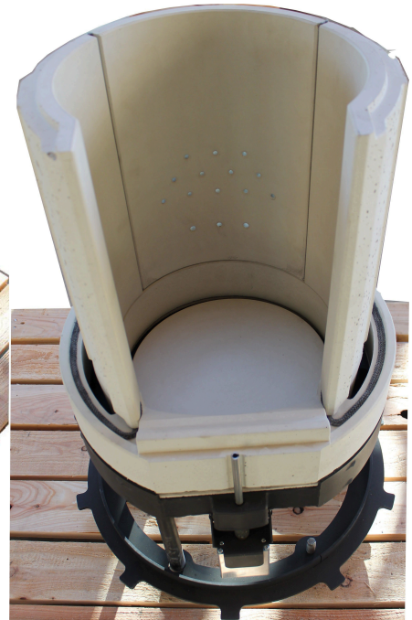
Illustration 16: Completed combustion chamber wall
