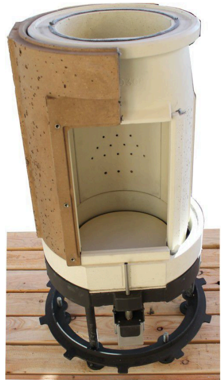
Illustration 18: Front inner ring and external shell, left side in place
